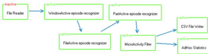
Figure 5: A module-setup in the ECG Lab used to investigate programming strategies in pair programming
